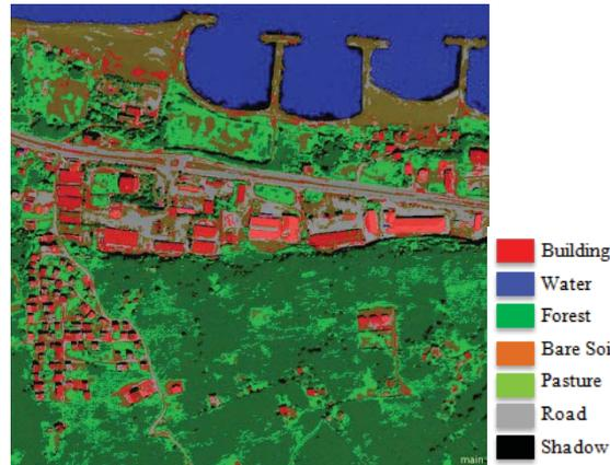
**Figure 3:** Result of image classification for optimum parameter (Scale=20, Shape=0.1, Compactness=0.5).
