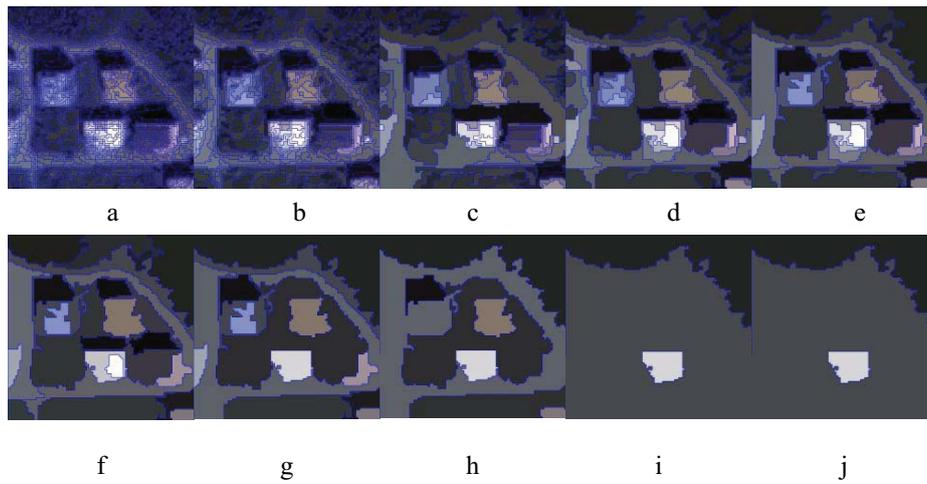
**Figure 2:** Segment sizes with different scale parameters (a=5, b=10, c=20, d=35, e=50, f=70, g=100, h=150, i=200, j=300).
