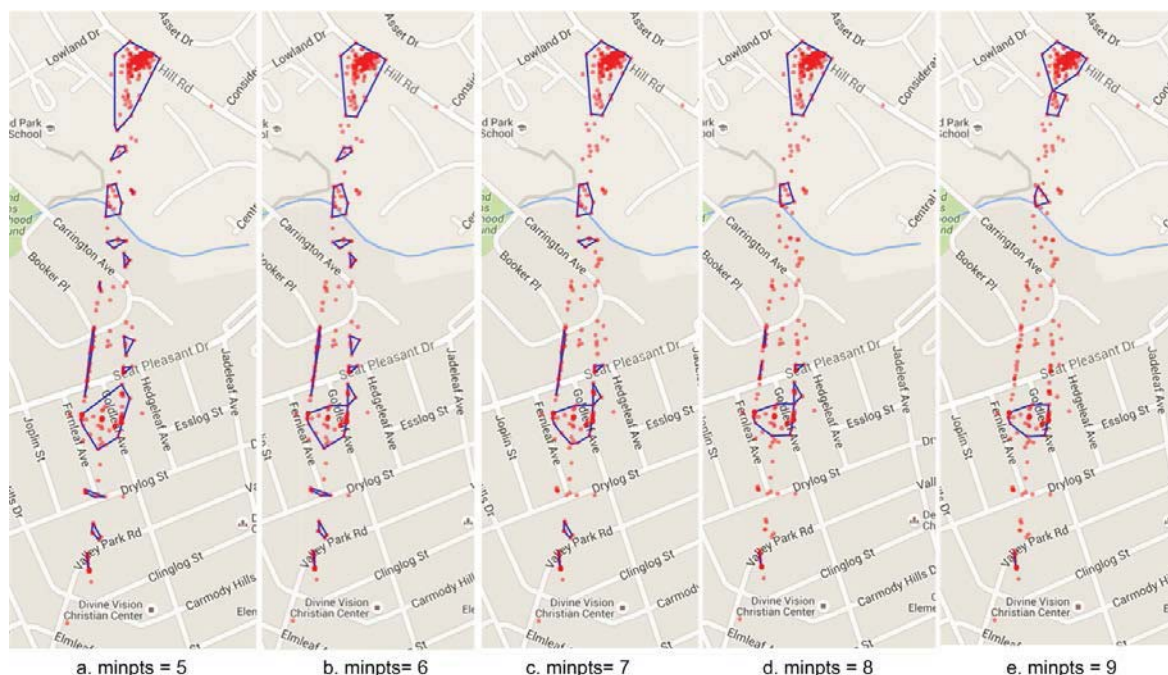
Figure 2: Detected clusters using different minpts values and a fixed eps value of 20 meters on dispersed locations (The geo-tagged tweets are displayed as red dots and the boundary of a cluster is depicted in blue)
