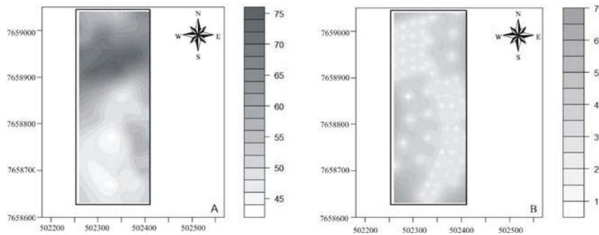
**Figure 3:** Kriging maps of the clay data (A) and standard deviation (B).
