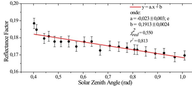
**Figure 1:** Graph of surface  $RF$  as a function of the solar zenith angle to the second band of the radiometer CE313/CIMEL, which ranges 595-701 nm. In red can be seen the function fitted to experimental data.
