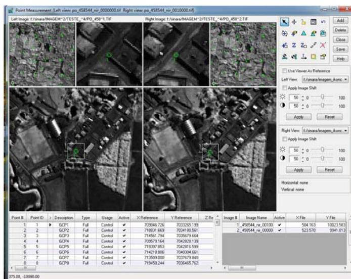
Figure 8: Currently LPS window add the GCPs (control points).
