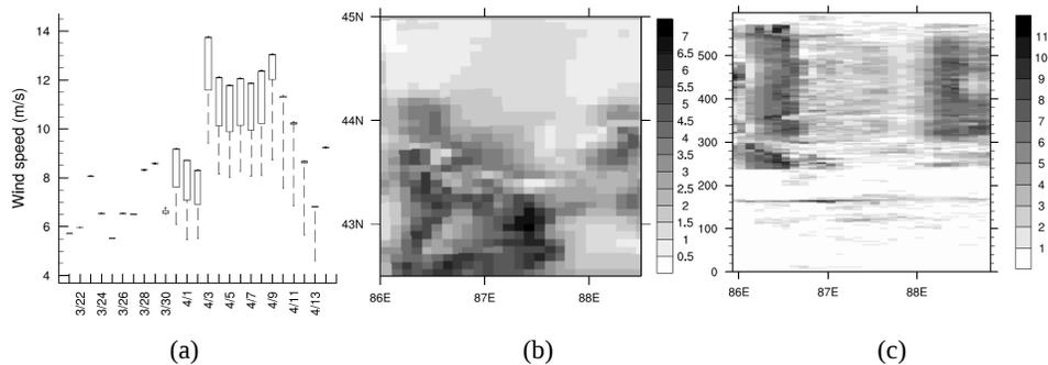
**Figure 2:** Uncertainty propagation illustrations for wind speed at 10 m above land surface: (a) aggregated temporal profile, (b) spatial profile of output ranges, and (c) spatio-temporal profile of output ranges along 44°N at hourly resolution.
