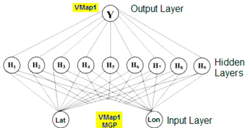
Figure 1 Layers implemented in the Artificial Neural Network (VMap1/MGCP data as Input and VMap1 as output).
