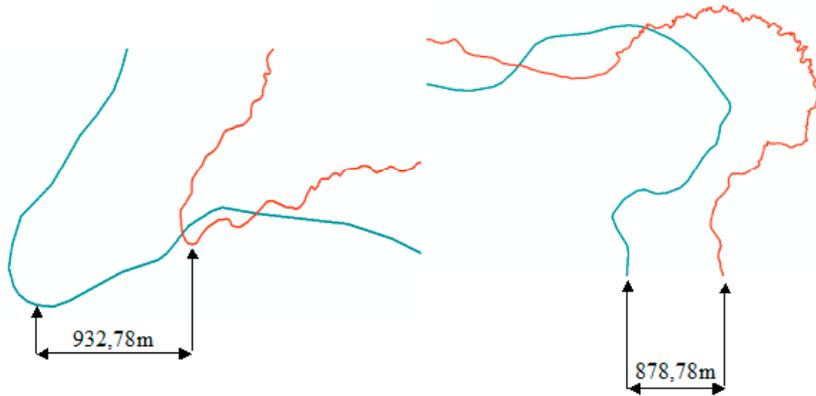
Figure 3 Differences obtained from S. Vicente Island boundaries of VMap1 (in blue) and MGCP (in red).
