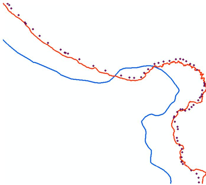
Figure 7 Application of the best neural networks achieved in Latitudes and Longitudes for the Boundary's theme. In blue the original VMap1 Boundary, in red the MGCP Boundary theme, and the points are the result of the transformation done by the neural network of VMap1 Boundary points.
