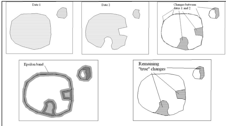
Figure 2 Detection and deletion of false polygons of change.
