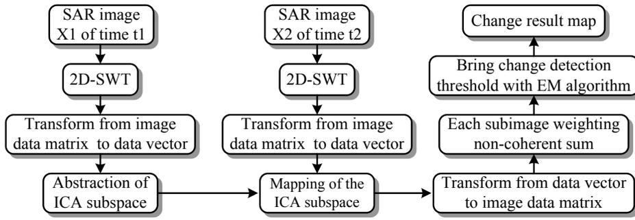
Fig. 1 The flow chart of SAR image change detection algorithm based on ICA and wavelet transform
