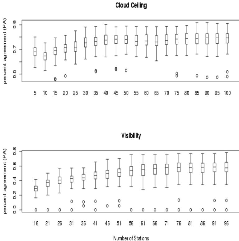
Figure 5: *PA for predicting the event of poor visibility for cloud ceiling height ( $n = 5, 10, 15, \dots, 100$ ) and visibility ( $n = 16, 21, 26, \dots, 96$ ) for the entire New England subset from nested designs. Only the ten nearest neighbors used for prediction with design sizes greater than or equal to ten.*
