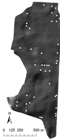
Figure 2. The digital elevation model with 2 m grid size created from GPS measurement. The white spots were the locations of soil samples used for model development
