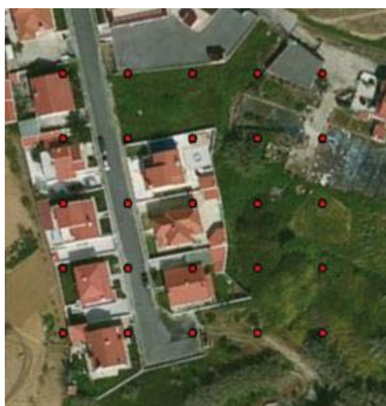
Figure 2: Example of SSUs organised in a 5x5 20m grid
